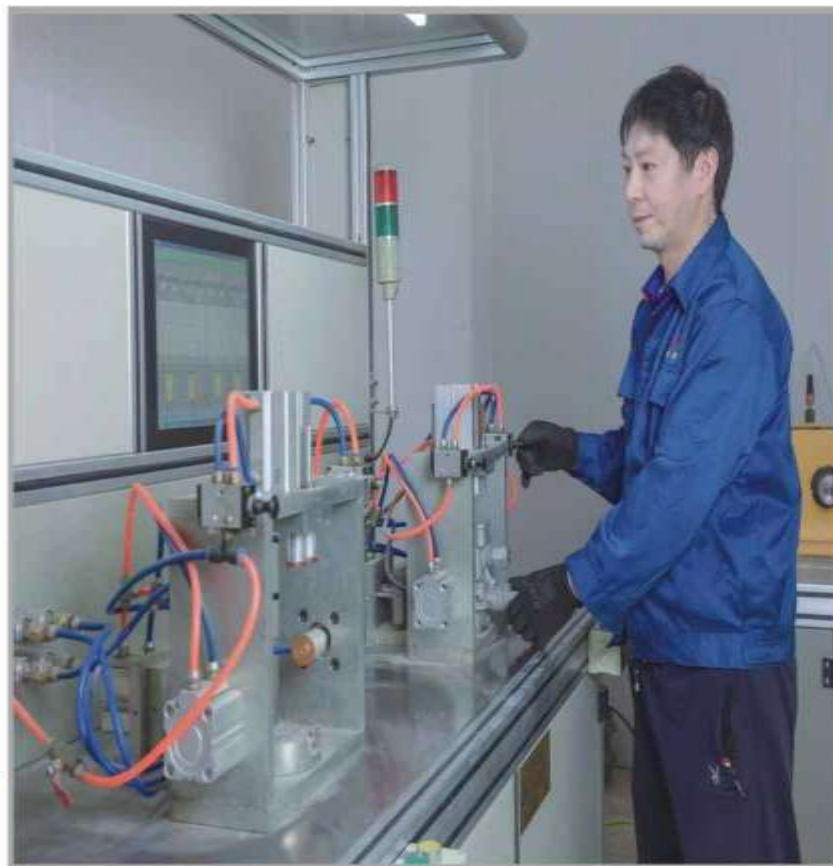
Air Valve Performance Test Equipment
